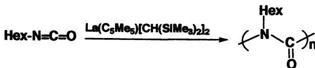
Fig. 8. Living polymerization of alkyl isocyanate
